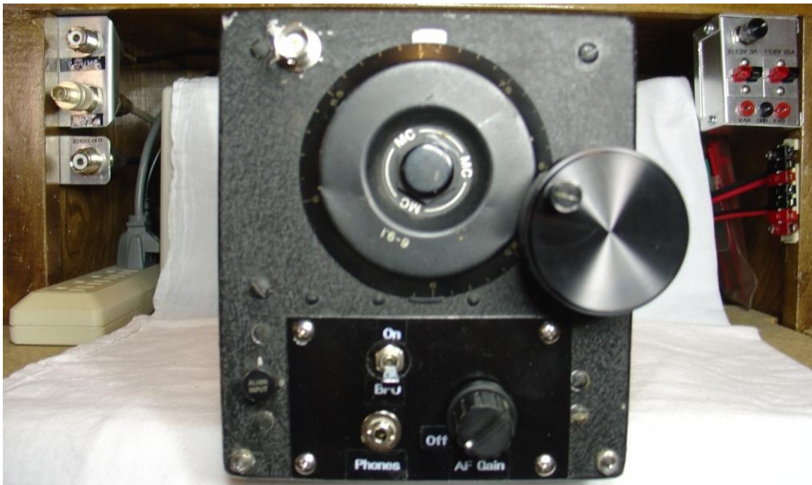
Figure 13: New tuning knob in place on author’s BC-455
