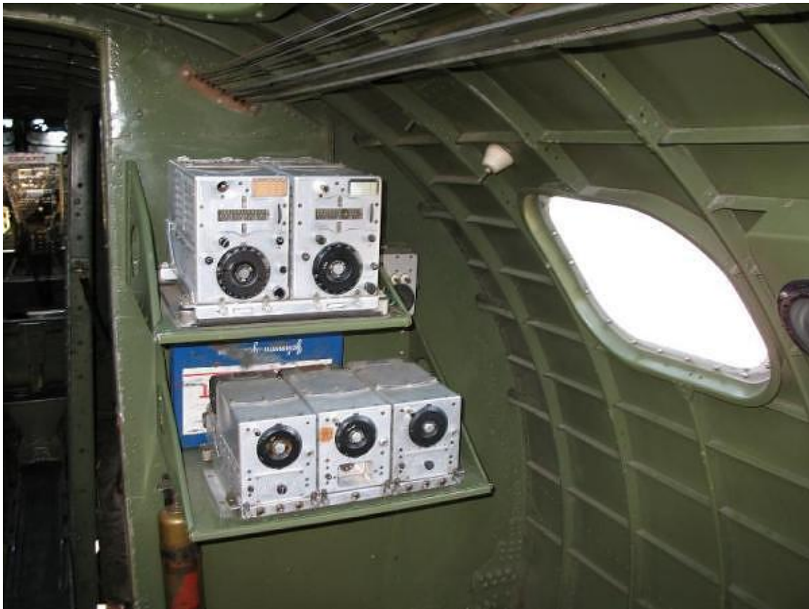
Figure 1: ARC-5 Equipment in a B-17 Bomber
