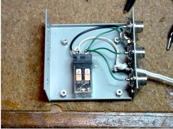
TR Switch – Inside Wiring
