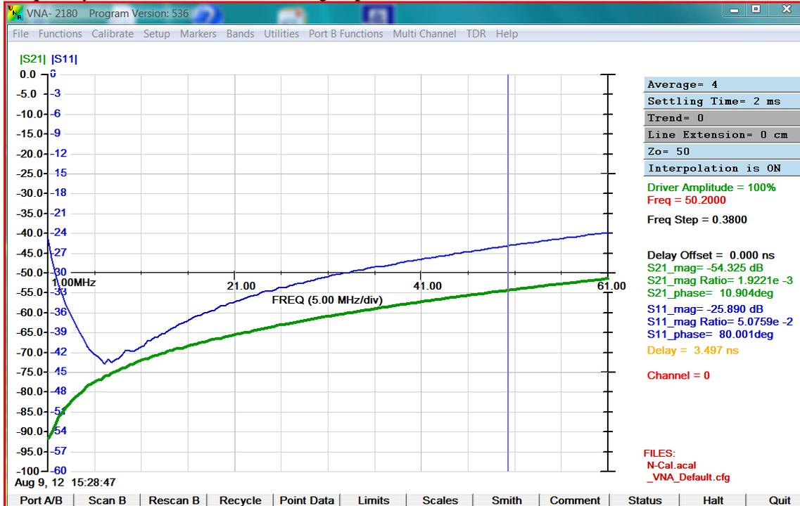
Figure 5: Port 1-2 isolation (green) and port 1 return loss (blue)
