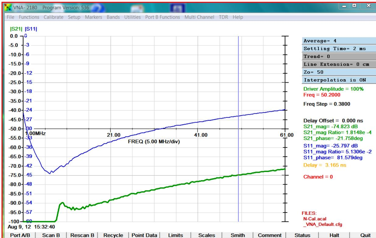
Figure 6: 1-3 isolation (green) and port 1 return loss (blue)
