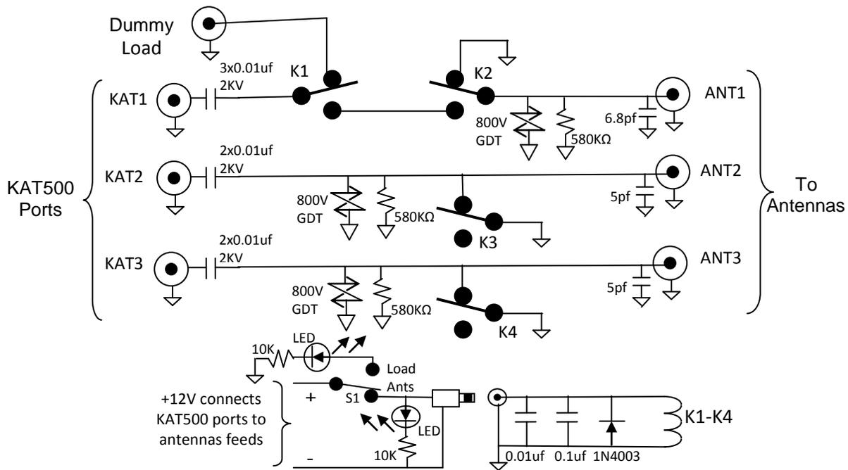
Figure 1: Schematic - Coax Feedline Protection and Management Box
