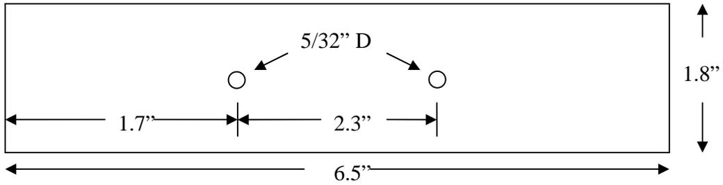
Figure 1: Battery Mounting Plate Dimensions
