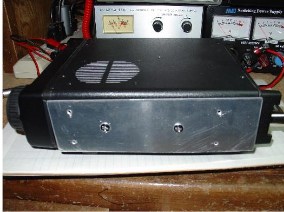
Aluminum plate mounted on IC-703
