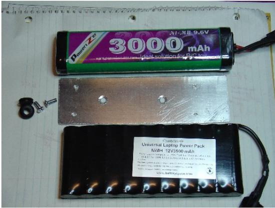
9.6V battery (top), parts (center), 12V battery (bottom)
