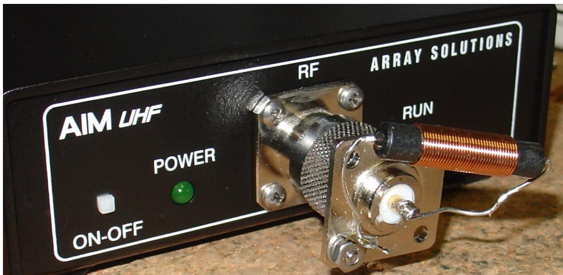
Figure 2: Inductor test set-up
