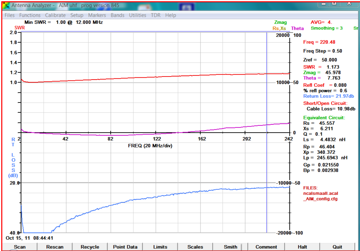
Figure 8: Bias-T SWR with compensation
