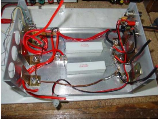
Wiring w/o switches and 2Ω resistors
