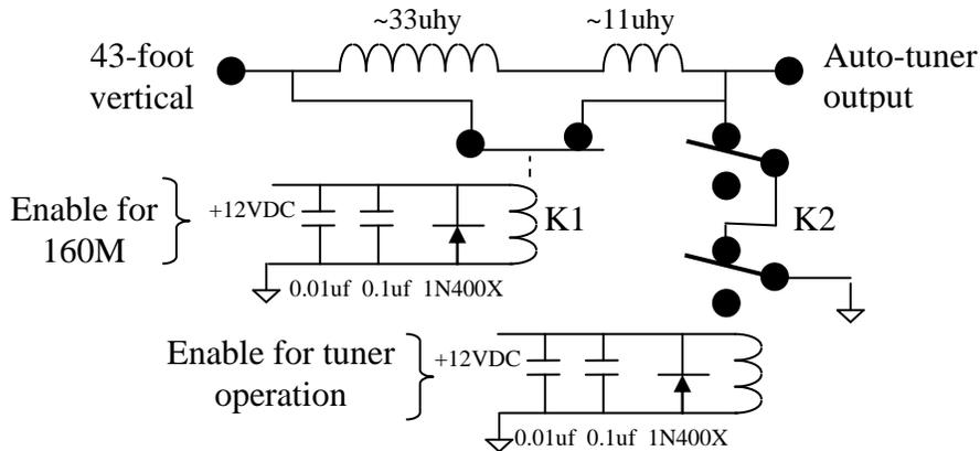
Figure 4: Remote switchable range extender/tuner protector
