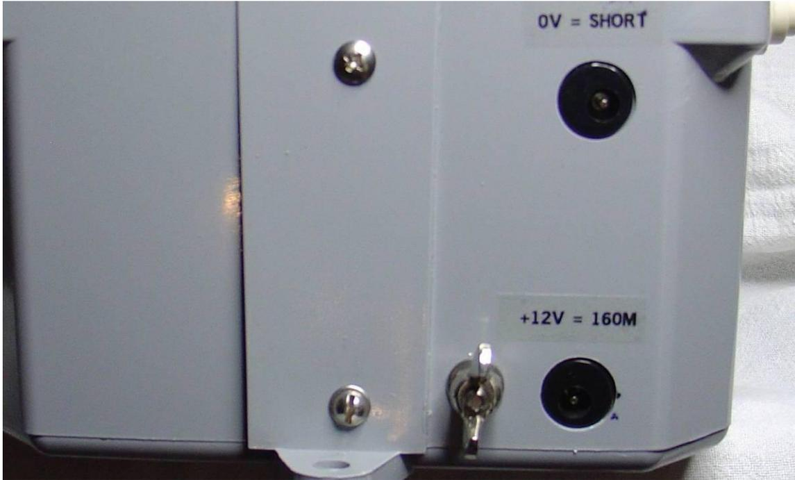
Figure 6: Auto-tuner Range Extender/Protector DC control jacks
