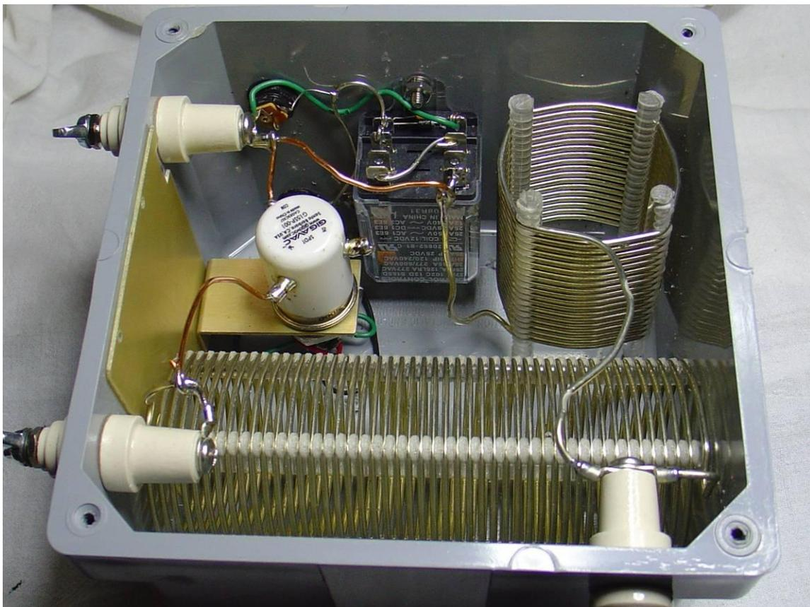
Figure 5: Gigavac 15KV relay (left), and RF-10 relay (middle) installed in extender.
