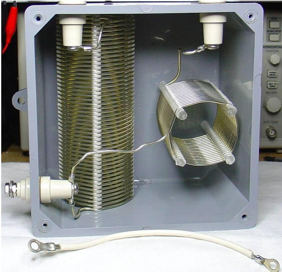
Figure 2: Inductor assembly internal view and shorting cable for 160M,
