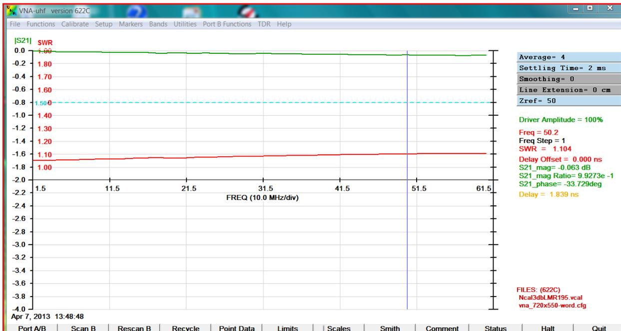
Figure 7: Transmit path SWR and insertion loss
