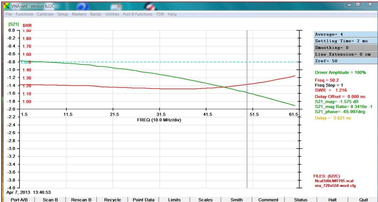
Figure 8: Receive path SWR and insertion loss
