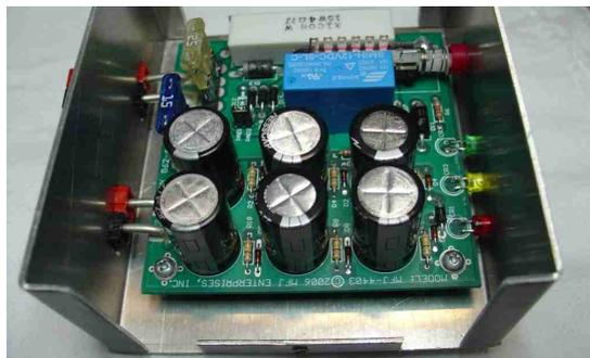
Photo F: Six 25-farad capacitors in series!
