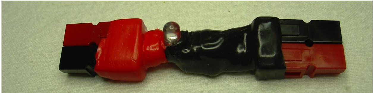
Figure 3: Completed reducer assembly. Battery connects to right side, and radio to left side.
