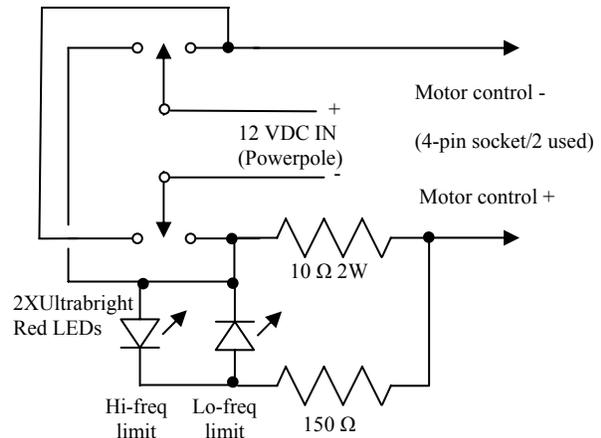
Figure 1 – Direction control and limit indicator
