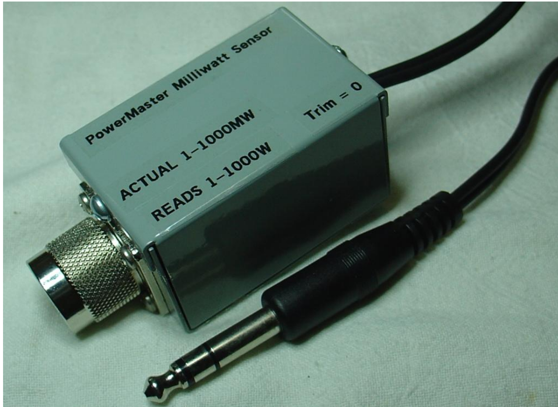
Figure 7: Completed Milliwatt Sensor. Only a mono plug/cable is necessary (see text).
