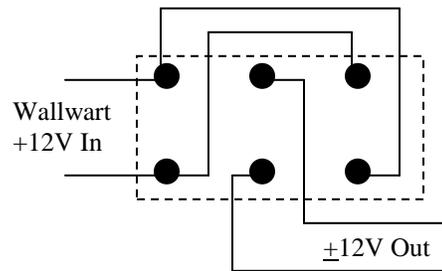
Figure 12: Physical Switch Wiring
