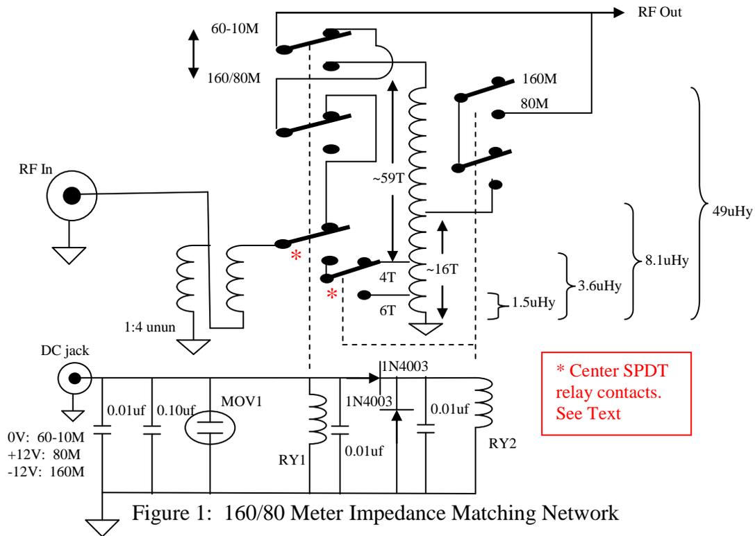
Figure 1: 160/80 Meter Impedance Matching Network
