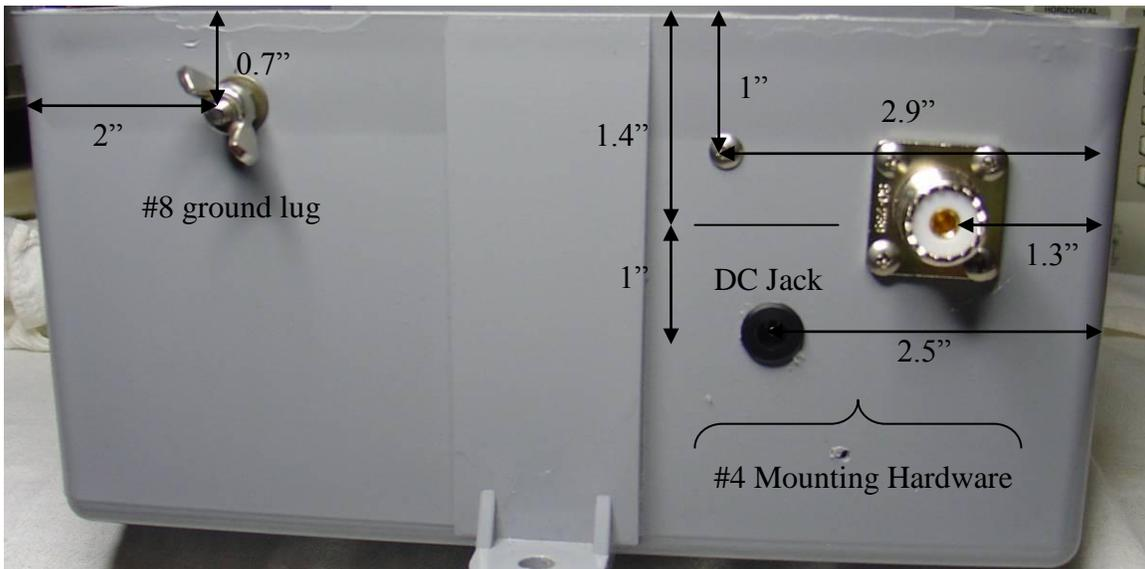
Figure 5: Ground, terminal strip, DC and RF mounting locations
