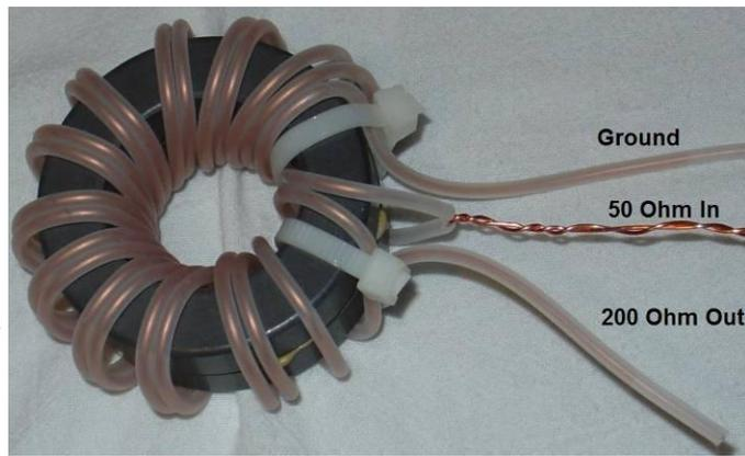
Figure 10: Voltage Unun (MFJ 10-10989D shown)
