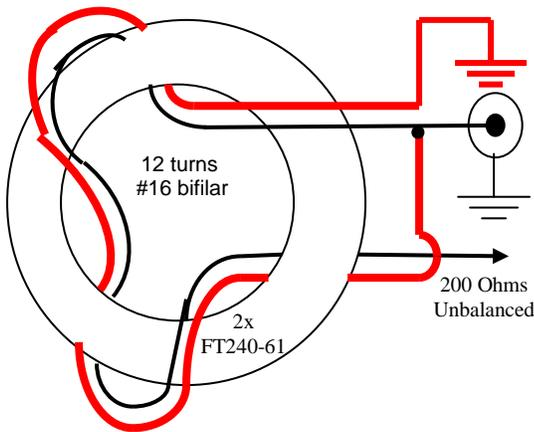
Figure 9: Voltage Unun Wiring
