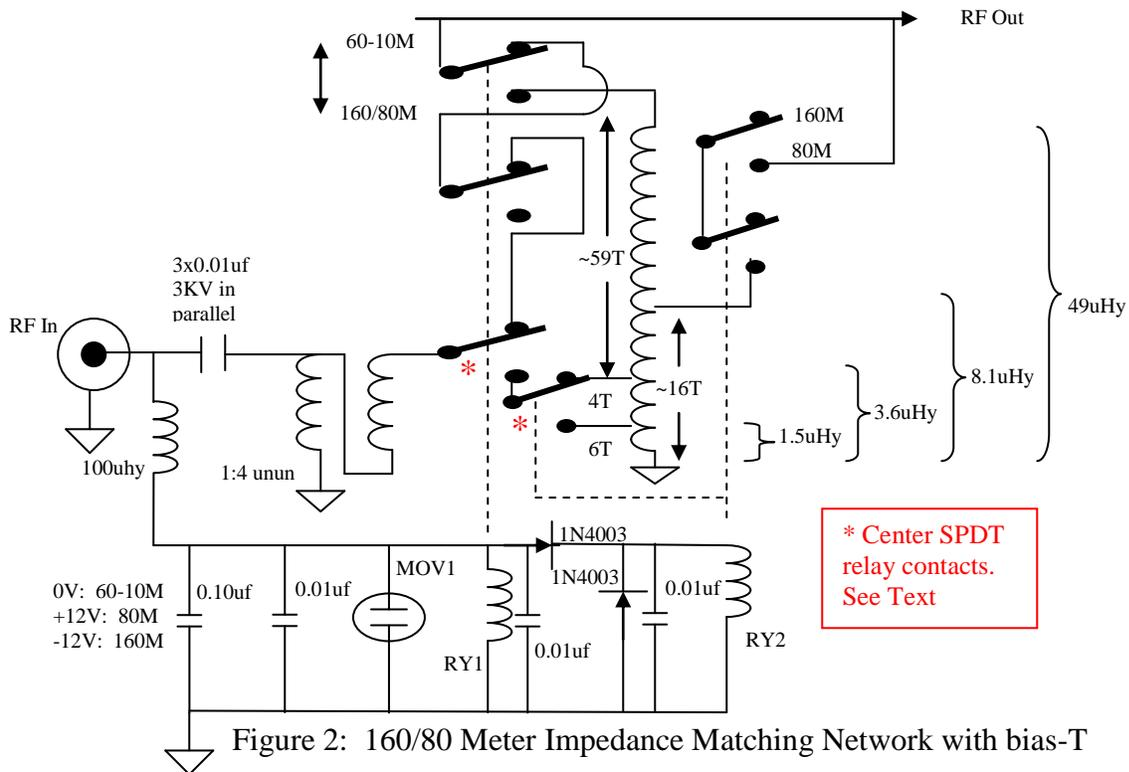
Figure 2: 160/80 Meter Impedance Matching Network with bias-T
