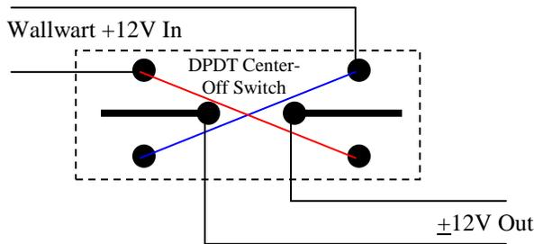
Figure 11: DC Switch Schematic
