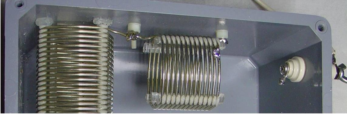
Figure 6: Hot glue and nylon-screw supports for the two coils
