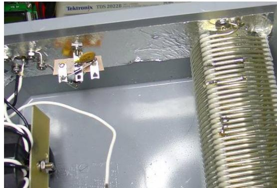
Figure 4: AL tape, term strip, & coil ground
