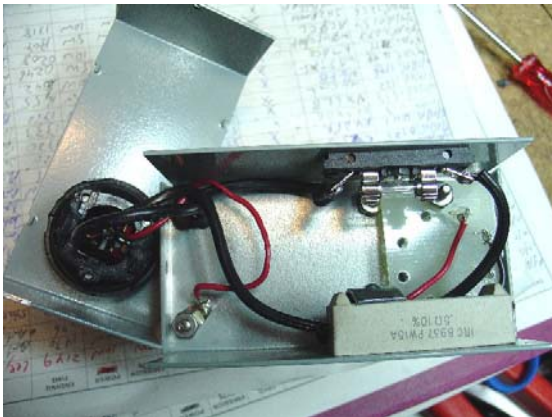
Inside Wiring of Night-Light
