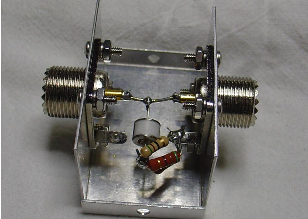
Figure 3: GDT transmitter limiter ready for test
