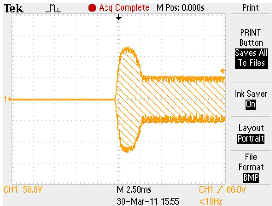
Figure 1:  $V_{pk} \approx 115V$ . PowerMaster peak power measured = 132 watts.
