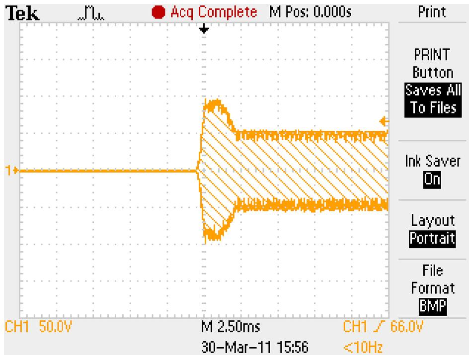
Figure 4:  $V_{pk} \approx 85V$ . GDT/ $16\Omega$  resistor. PowerMaster peak power = 73 watts.
