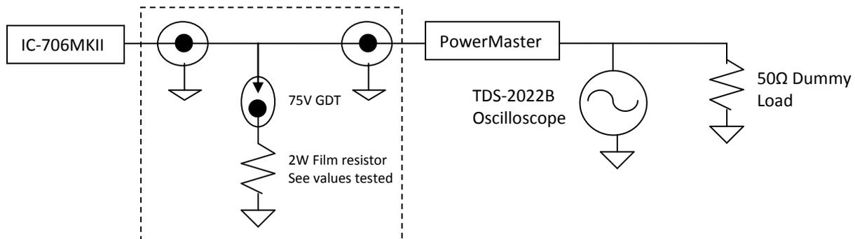
Figure 2: GDT Test Circuit
