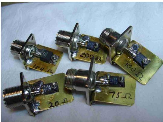
Photo B: Completed precision mismatches
