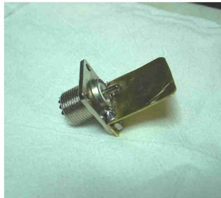
Photo A: Connector/Plate assembly
