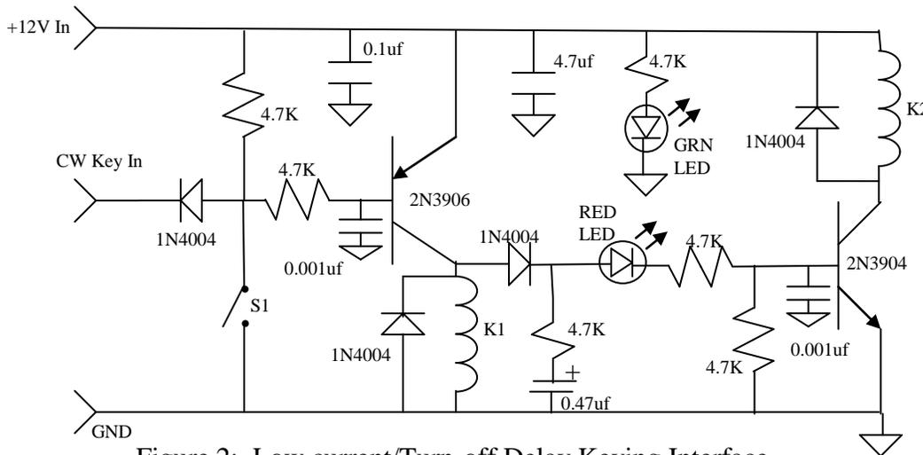
Figure 2: Low current/Turn-off Delay Keying Interface
