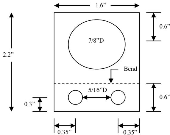
Figure 2 – Vacuum Switch Mounting Bracket
