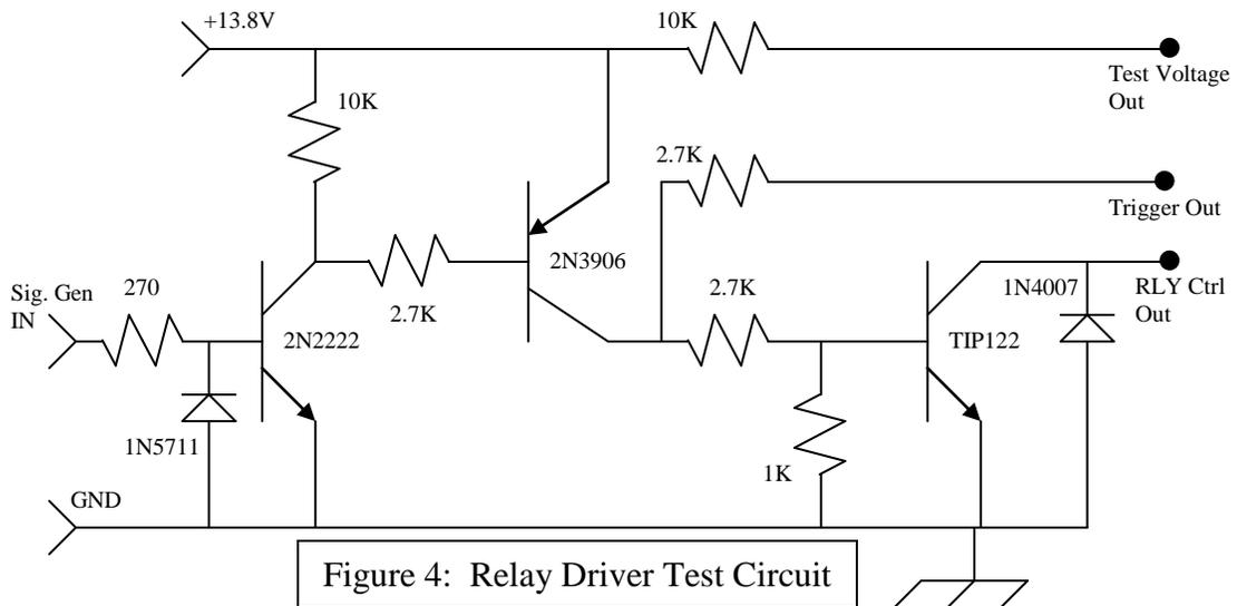
Figure 4: Relay Driver Test Circuit
