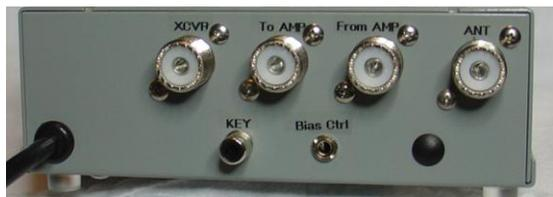
Photo F: Rear view of the QSK switch.
