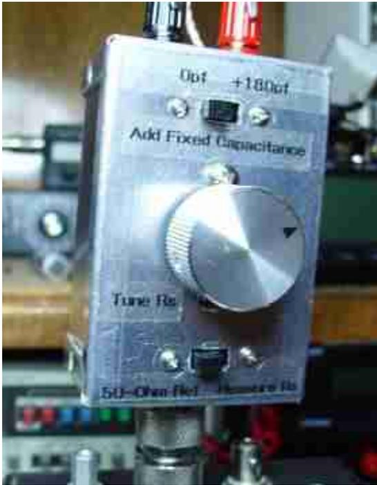
Photo B: Q-Adapter front panel
