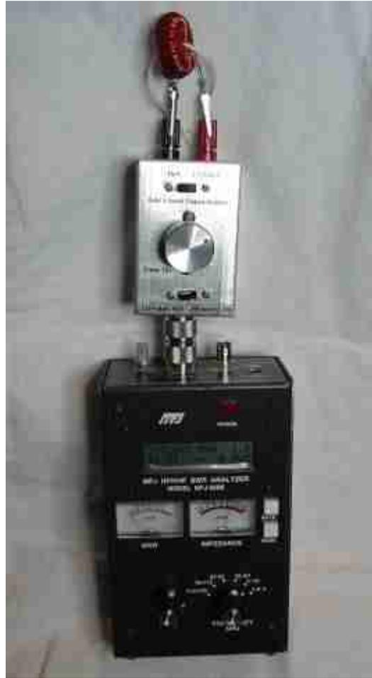
Photo C: Measuring inductor  $R_s$
