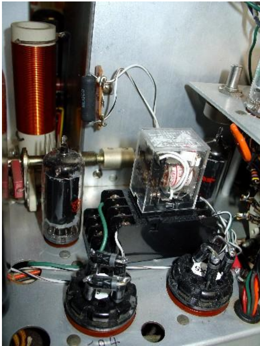
VFO resistor, Relay, and Rectifiers
