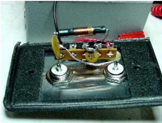
Photo C: DC Out (internal view)
