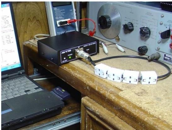
Photo E: AIM4170 Impedance Measurement
