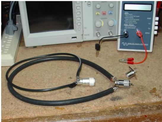
Photo C: Ferrite choke measuring loops
