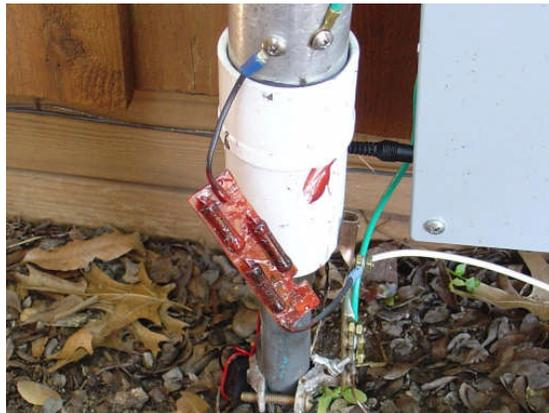
Photo B: 3x3MΩ in series on perf-board at base of author's 43-foot vertical
