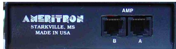
Amplifier interface cables connect to these ports on the rear of the ARI-500.
