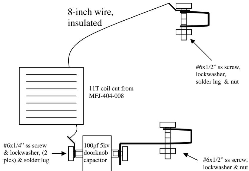
Figure 2: Trap Construction Details
