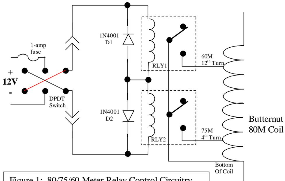
Figure 1: 80/75/60 Meter Relay Control Circuitry
