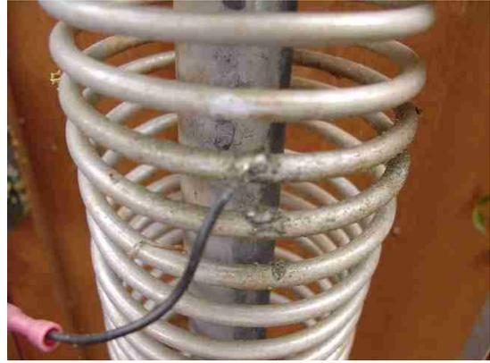
Photo 4: 60 meter soldered connection
