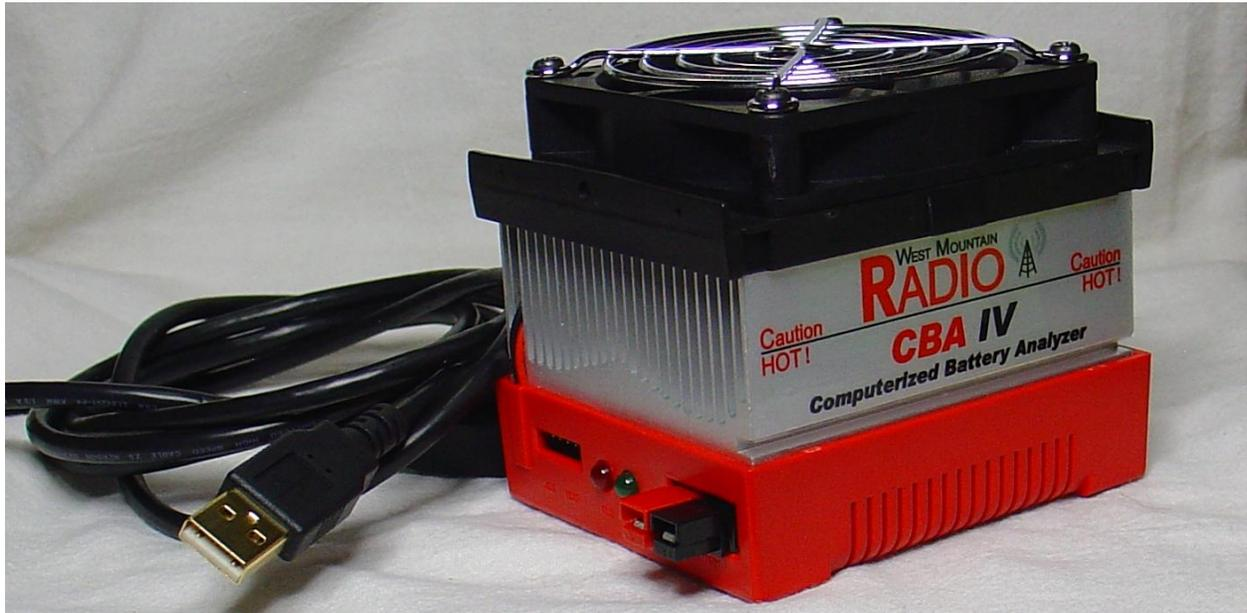
Figure 1: West Mountain Radio CBA-IV Battery Analyzer
