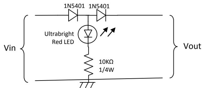
Figure 6: LiPo 4S Voltage Reducer
