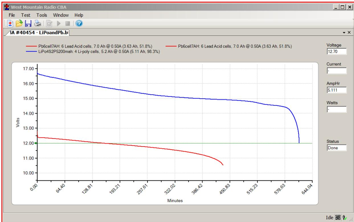
Figure 4: LiPo & Lead-acid Battery Testing showing minutes of use at 500ma average current
