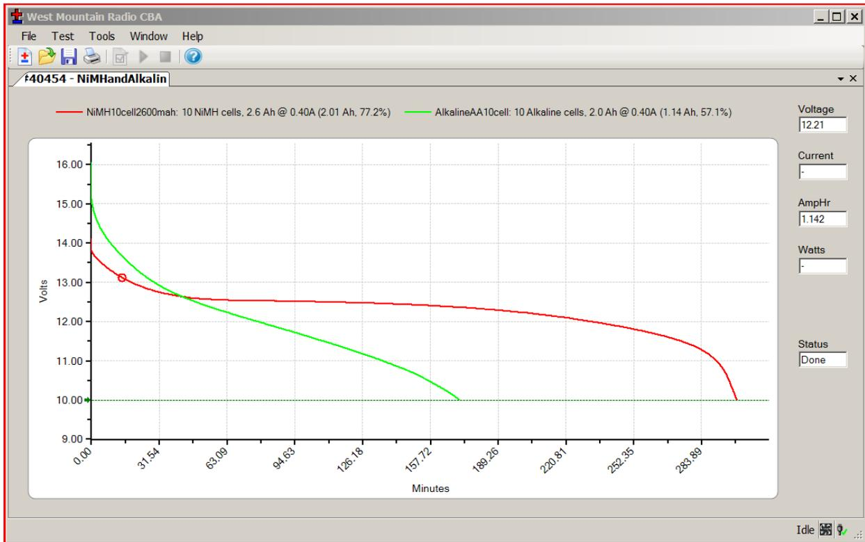
Figure 5: NiMH and Alkaline battery test results at 400ma average current
