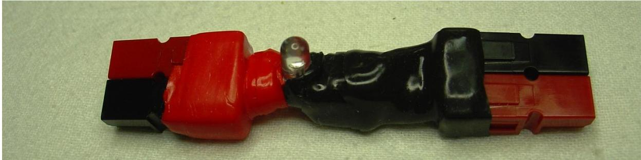
Figure 8: Completed reducer assembly. Battery connects to right side, and radio to left side.
