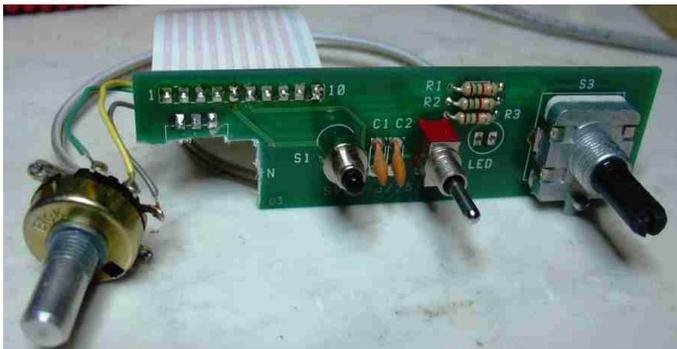
The nibbled area clears some of the pot protrusions, but you still need to mount the pc board a little farther back from the front panel to ensure clearance, and still keep the front panel parallel to the PC board. To do this, I found additional nuts for the encoder, freq, and keyer controls (washers would also work). I installed these nuts on the controls so the front panel would be about 0.1 inch further from the pc board. The photo below shows the front panel mounted with the new pot/switch.
