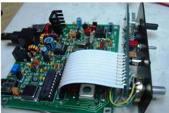
Next, flip over the main board and cut the circuit trace between the center pin of the DC power connector and the reverse protection diode. Then solder wires from the switch on the new pot to the power connector center pin and the reverse protection diode.
