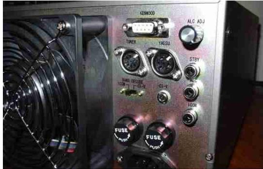
Photo D: Close-up of XCVR interfaces
