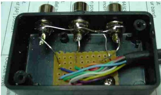
Photo E: IC-706 interface internal wiring
