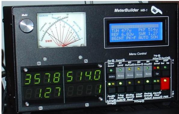
Meterbuilder MB-1 displaying average power, peak power, SWR & coupler selected.
