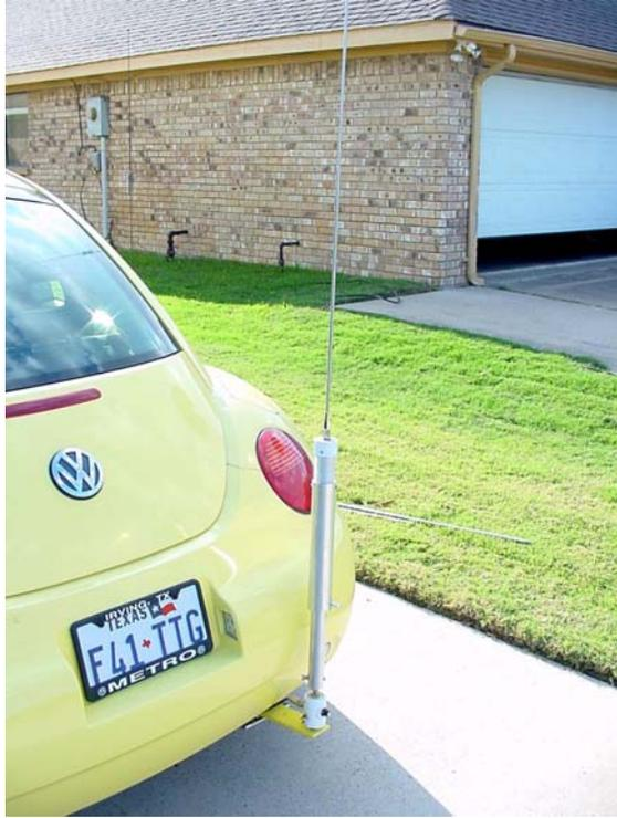
MFJ-1664 mounted on VW New Beetle
