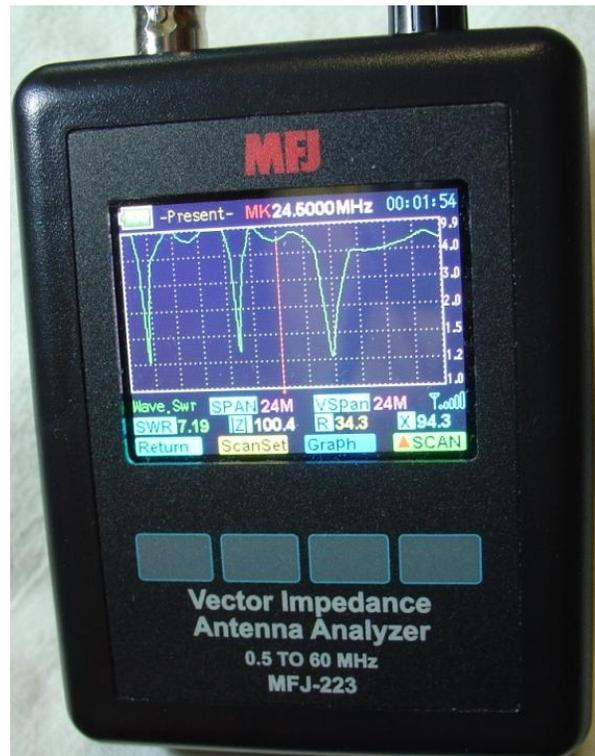
Figure 4: 20/15/10M trap dipole scan
