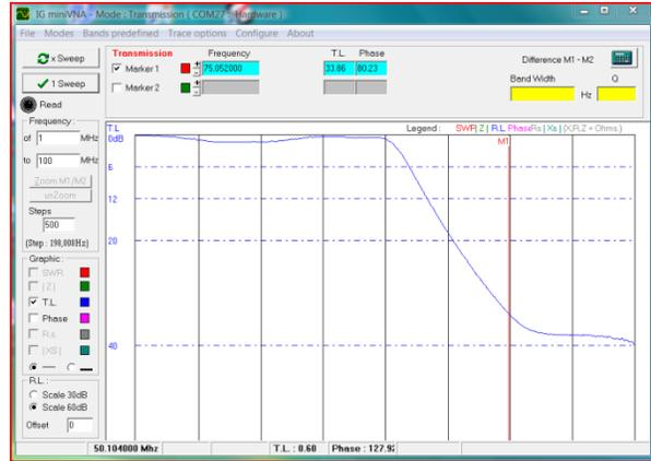
Figure 4: SWR/Return Loss plot of a 6M filter      Figure 5: Insertion loss plot of the 6M filter
