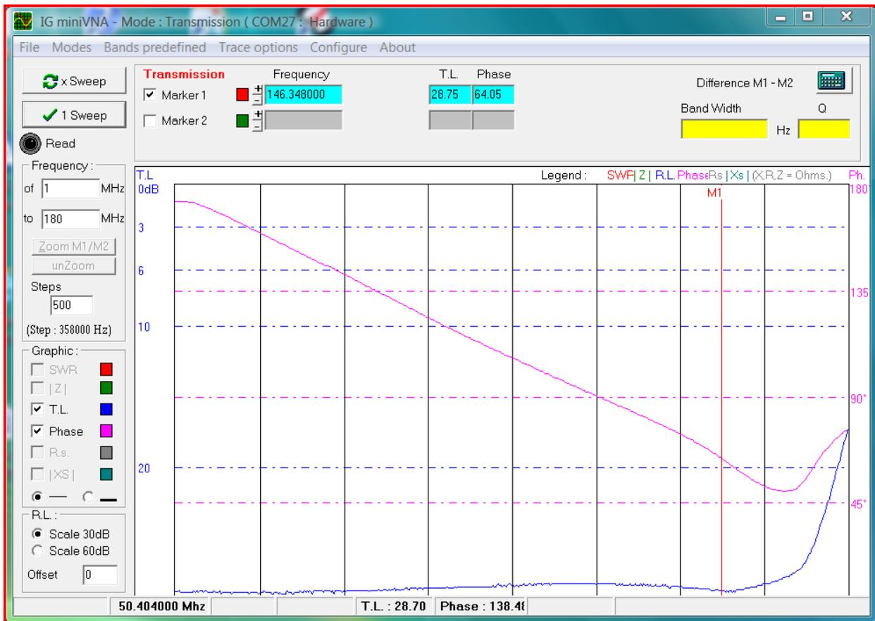
Figure 7: Attenuation of precision 30dB attenuator
