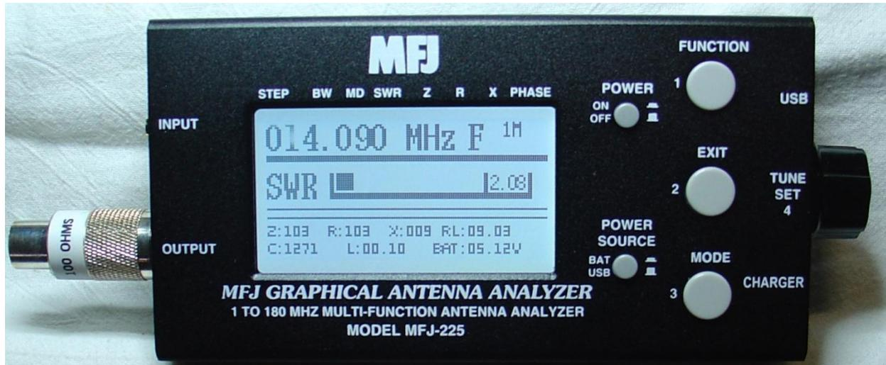
Figure 2: Single-frequency (ANT-G) mode measuring a 100Ω load
