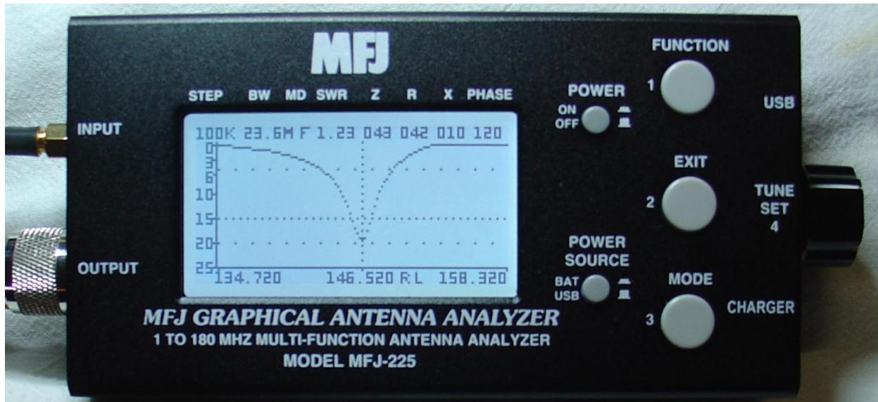
Figure 3: Return loss sweep of a 2-meter bandpass filter
