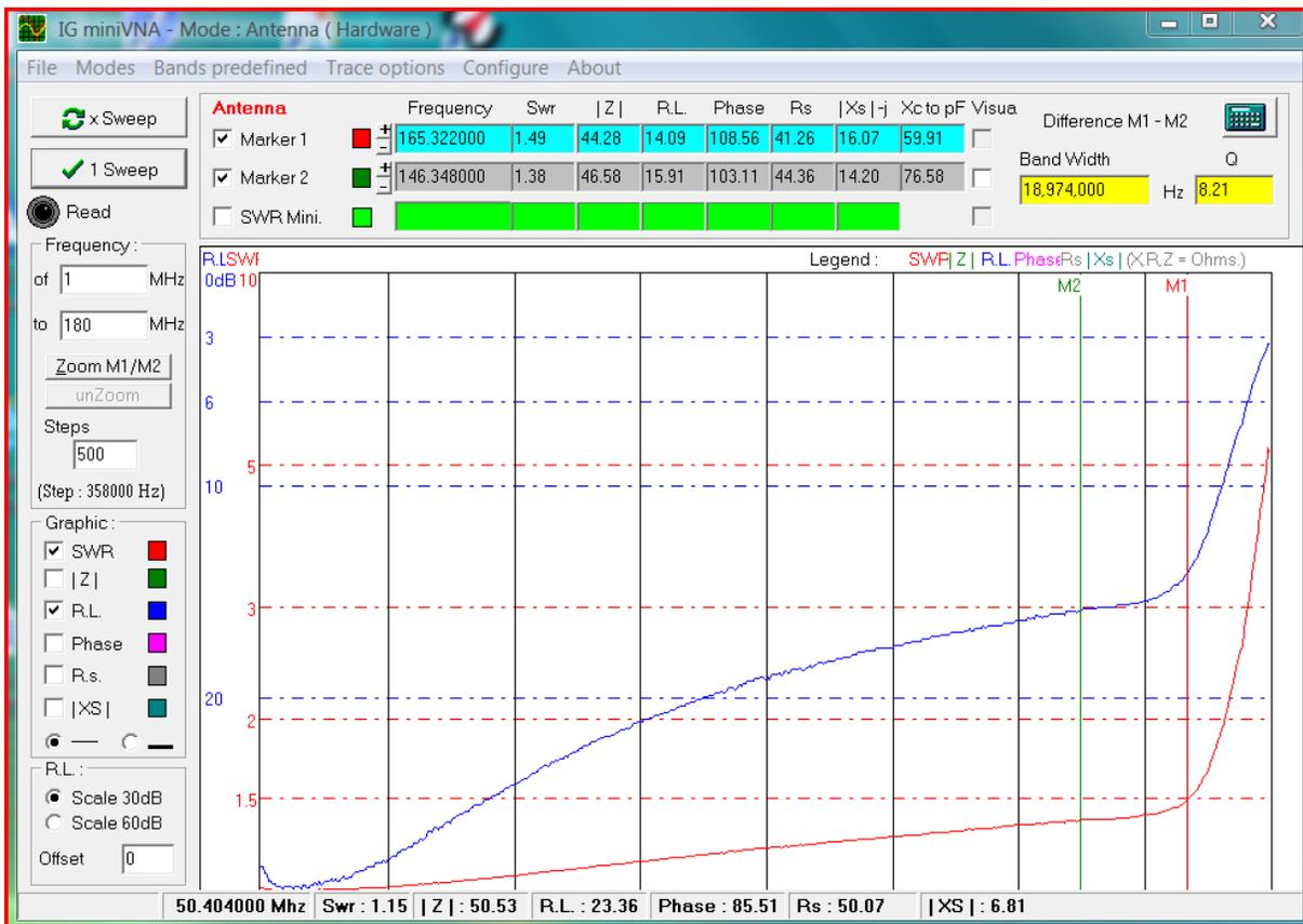
Figure 6: Precision 50 ohm load as measured by the MFJ-225 and IG-miniVNA software.
