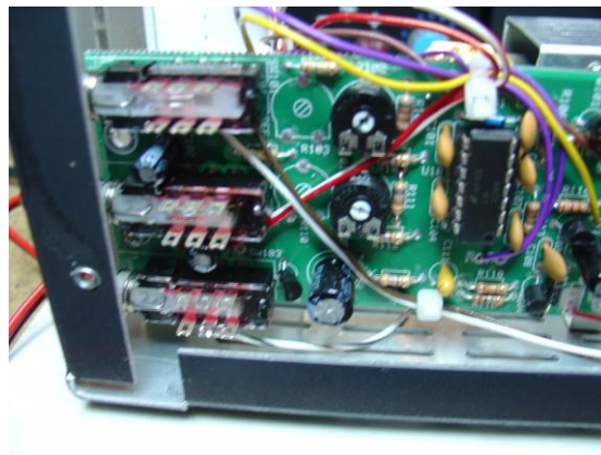
Photo B: Fan +12V striped wire (bottom) soldered to bottom center switch terminal
