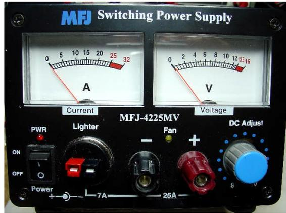
Powerpole plug assembly epoxied in place
