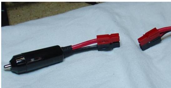
Photo D: Cut cable with PowerPoles
