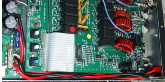
Photo G: New 14-gauge wiring
