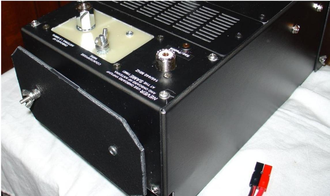
Photo K: New ground lug and stainless steel mounting screws on rear cover
