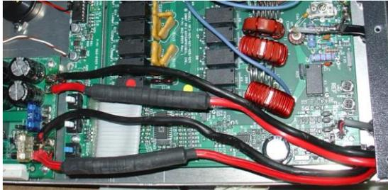
Photo F: Original 10-gauge DC wiring
