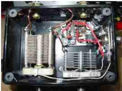
Internal SWR bridge mounting
