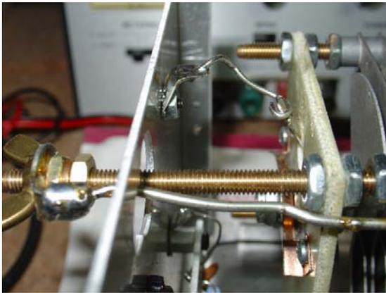
Antenna terminal interface to capacitor
