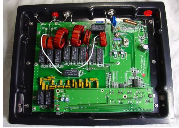
Figure 7: Internal view of the MFJ-994BRT
