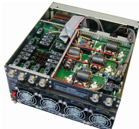
Photo C: RF section with shields removed
