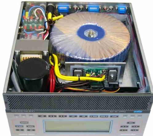
Photo B: Internal Power Supply (look at that power transformer!)
