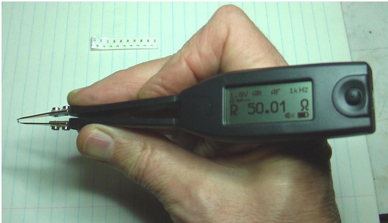
Figure 1: ST5 measuring a precision 0201 50-ohm SMD resistor
