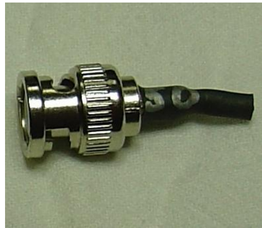
Photo B: Final BNC 50 ohm load
