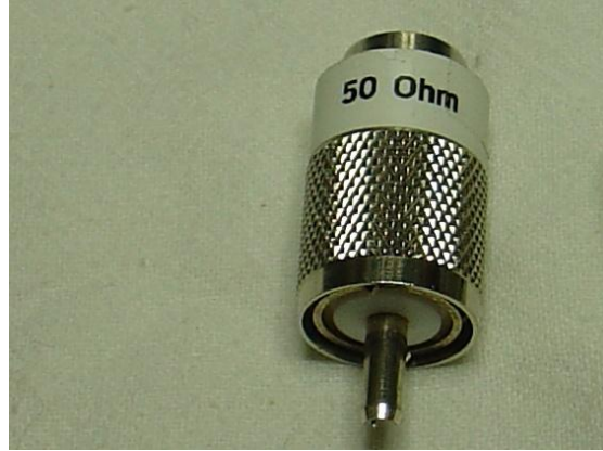
Photo C: PL259 and two 100 ohm resistors Photo D: Final 50 ohm load
