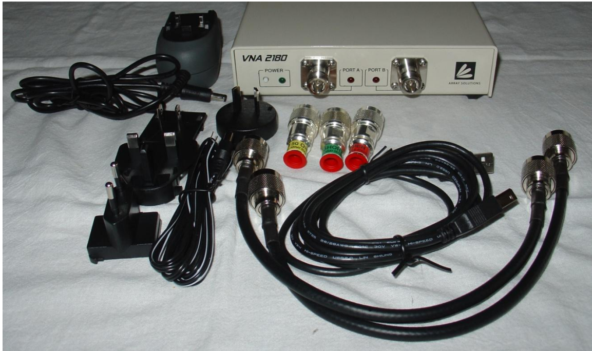
Photo A: Array Solutions VNA2180 Vector Network Analyzer & Supplied Accessories
