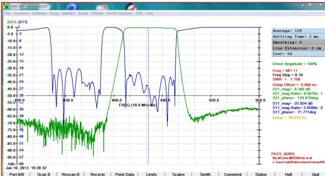
Figure 4: Cellular duplexer performance measured by the VNAuhf
