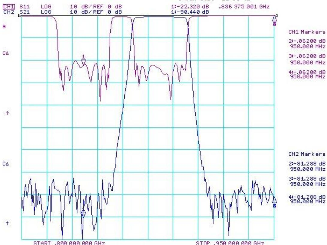
Figure 6: HP/Agilent 8722D measurement of the cellular duplexer
