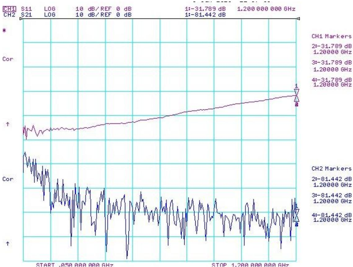
Figure 2: HP/Agilent 8722D measurement of Array Solutions precision 50 ohm load
