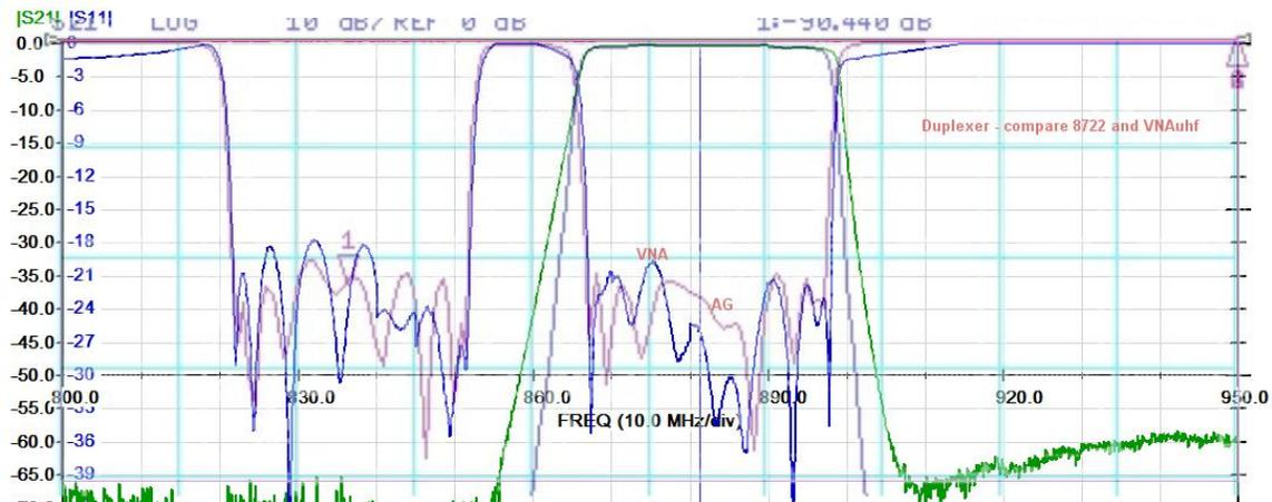
Figure 7: VNAuhf and Agilent 8722D performance overlay
