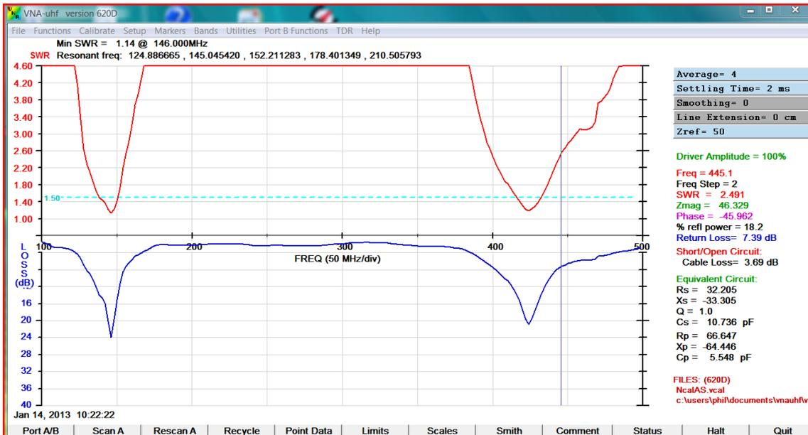
Figure 3: SWR and Return Loss evaluation of a 19" whip on both 2-meters and 3/4-meters
