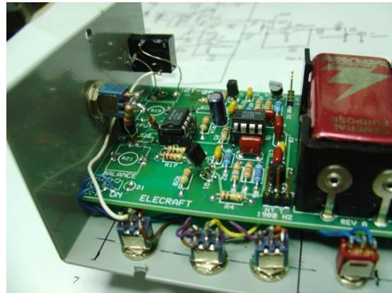
Photo F: 2T-gen mounted in aluminum box
