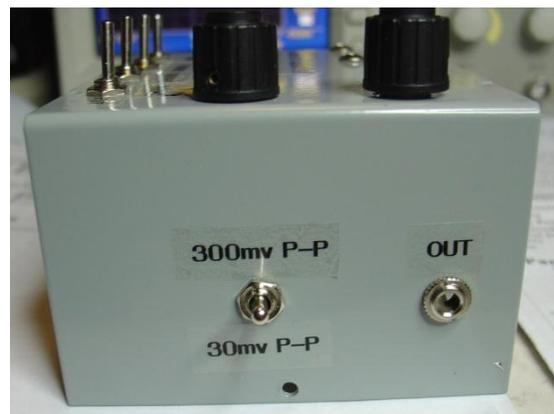
Photo H: Range control & output connectors
