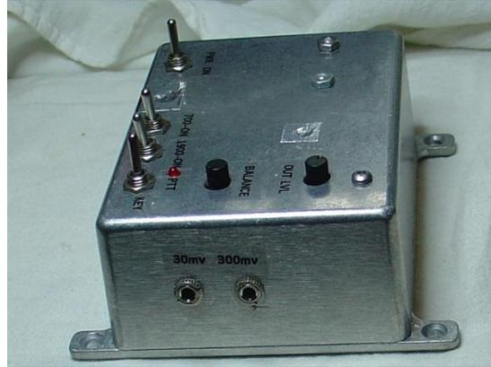
Photo J: Low- and High-Level outputs
