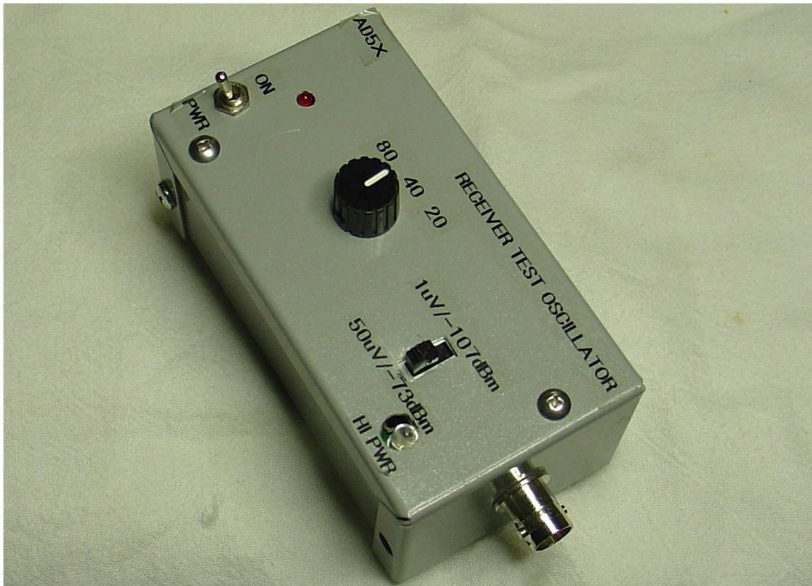
Photo D: Different view – better shows the BNC connector output.
